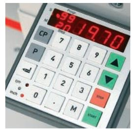
The "EP" back gauge control module stores 99 programs and frequently used measurements.
