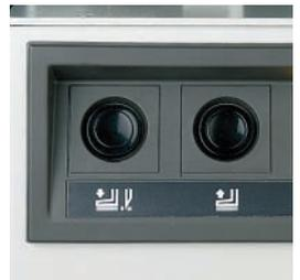
The automatic clamp control allows clamp to be moved up or down, independent of blade.
